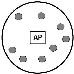
The above diagram shows a basic cell. Within the cell, each station can “hear” all of the others. In a more practical situation, not all of the nodes can “hear” all of the others. In this case, the cell must have a master controller, called the Access Point. The AP must be able to hear all of the nodes and coordinate all intra- and inter-cell traffic.
