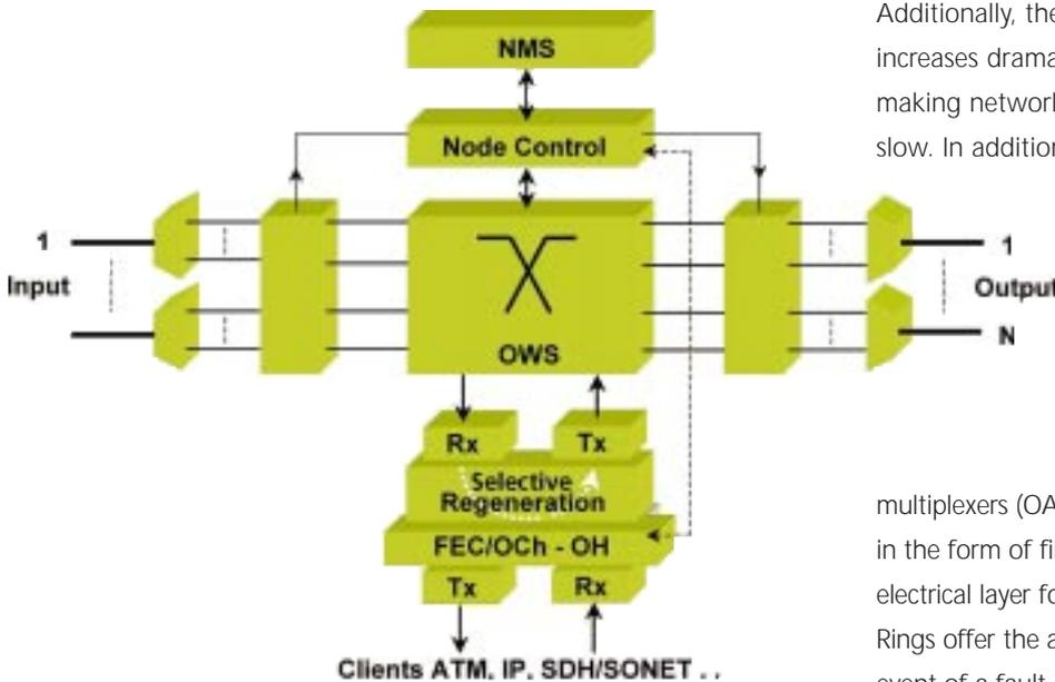
objectives. However, the influence of Internet infrastructure architecture has caused operators to reconsider mesh structures as a means of creating network resilience. Mesh structures call for optical cross connects (OXC) rather than the use of back-to-back OADM to create cross connect functionality.
