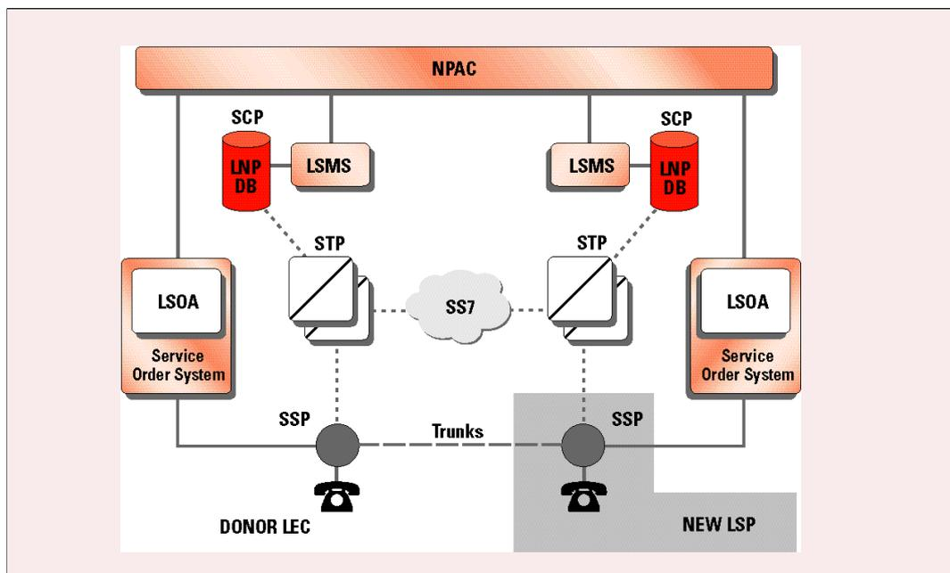
Figure 3 - Relationships of Carriers, Network Components, and LNP Systems with the NPAC
