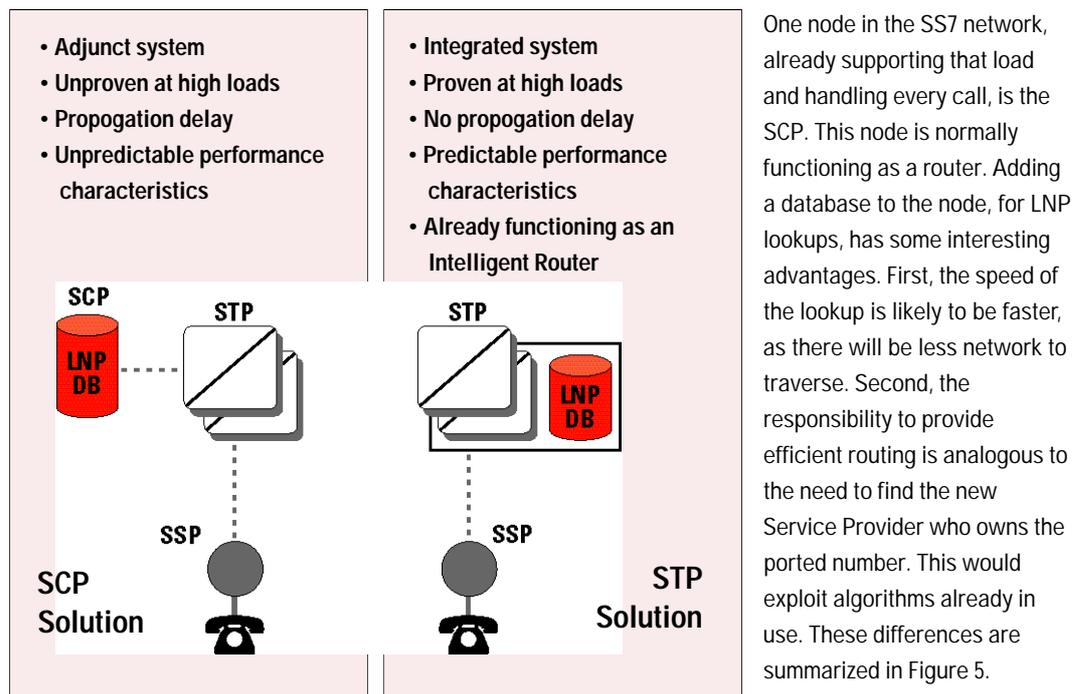
Figure 5 - Traditional SCP Solution vs. STP Solution
