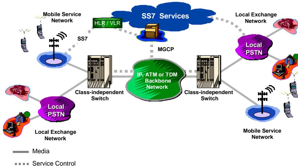
*Figure 3 — A converged solution for long-haul or tandem networks.*
