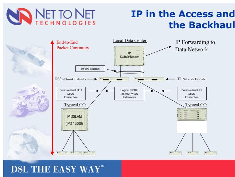
Figure 3 – DSL Solution using IP in the Access and the Backhaul
