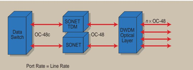
**FIGURE 3 CONNECTING ATM & IP DIRECTLY TO THE OPTICAL NETWORK**
